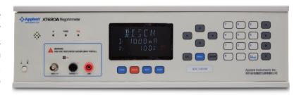
Power Supply 198VAC~240VAC 47.5Hz~52.5Hz Power: maximum 100VA
