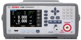
Power Supply 85VAC~250VAC 50Hz~400Hz Power: maximum 300VA
