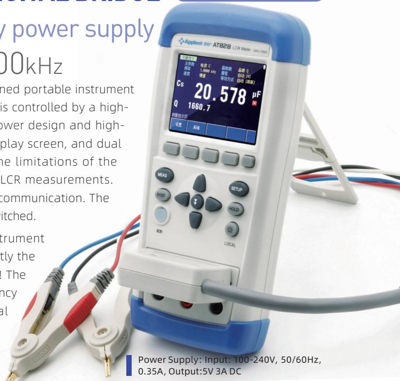
Power Supply: Input: 100-240V, 50/60Hz, 0.35A, Output: 5V 3A DC
